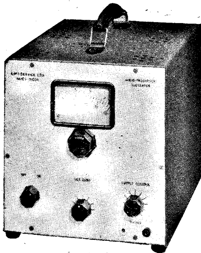
This E.M.I. Service audio oscillator provides signals for injection into any part of the AF section of a receiver.
